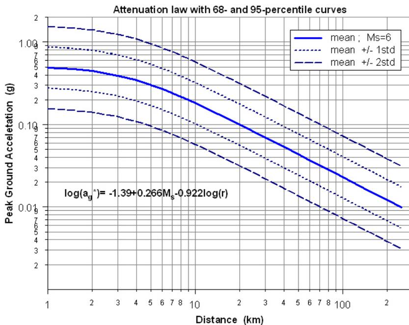
Fig. 4.3. Scatter of the predicted values of the peak ground acceleration for the attenuation relationship for the European area proposed by Ambraseys et al.[13-14].
