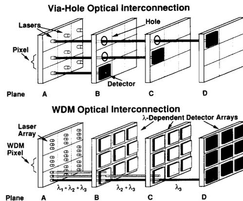
Fig. 1. 3-D view of one-to-many optical plane interconnections using (a) via holes which establish a permanent optical path, and (b) 2-D pixel array of identical 3- $\lambda$  VCSEL mini-arrays and three  $\lambda$ -selective detector arrays.
