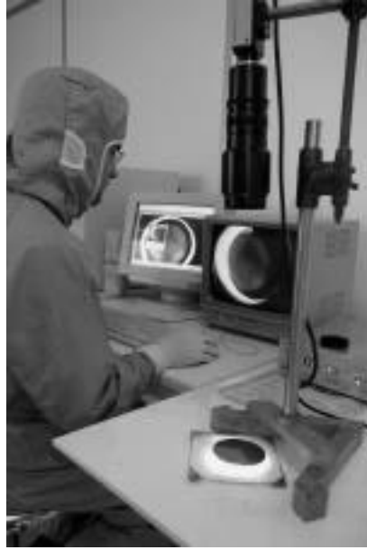
Figure 8. IR-camera inspection set-up.
